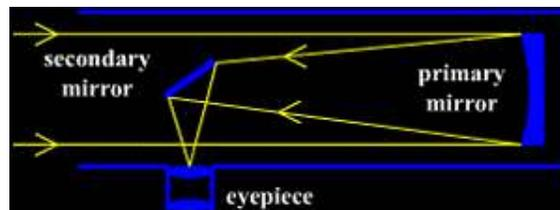
**The Newtonian reflector uses a concave primary mirror at the end of the tube which directs light back up to a secondary mirror and then on to the eyepiece. A Newtonian is usually cheaper to buy, inch for inch of aperture, than the other main telescope designs. Newtonians are good all-round workhorse telescopes suitable for all types of astronomical viewing and astrophotography.**
