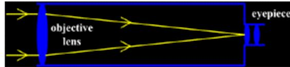
Refractors are what most people think of when they think of telescopes - light enters through an objective lens at one end and comes out of an eyepiece at the other. They are generally used for lunar and planetary work, and since they provide an upright image they are suitable for terrestrial observing. The tube is sealed and the objective lens is permanently set and aligned. Their simplicity of design makes them easy to use and maintain.
