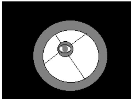
Fig 2. Small mirror adjusted. Primary mirror requires adjustment.
